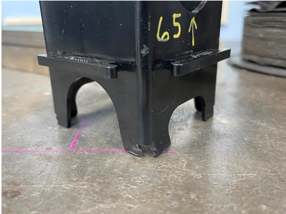
Typical Base Feet Failure
